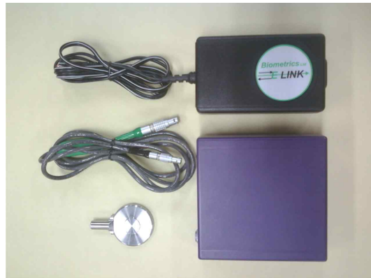
Fig 1. Electro Pinch meter G-100 (Biometrics. Ltd., UK)
