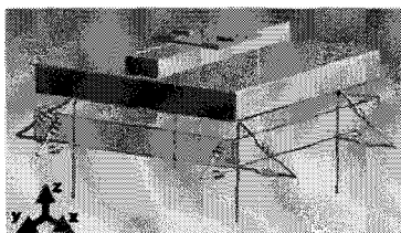
(c) 3rd Mode Shape( \omega_z )
