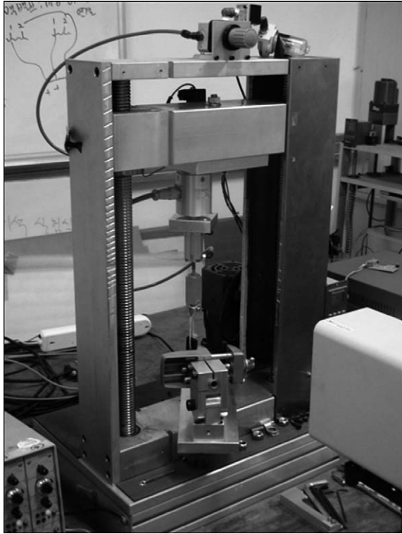
Fig. 3. The MTS Q Test/5 (Material Testing System, Eden Prairie, MN) and the laser extensometer were positioned for experiments.
