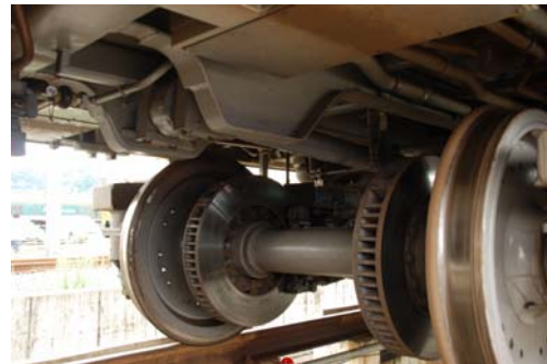
Fig. 8 A picture of disk brakes of the TTX tilting train
