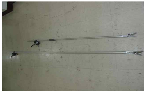
Fig. 4 Picture of high-ground trimmer improvement used in hydraulic system.
