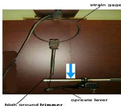
Fig. 6 Measuring of lever tension.
