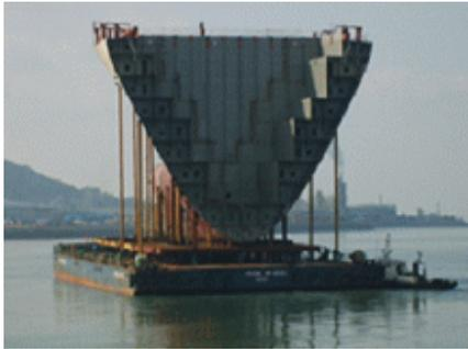
Fig. 1 An example of Fore body block transportation
