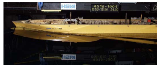
Fig. 5 Model test of optimized hull form at 24.0 knots
