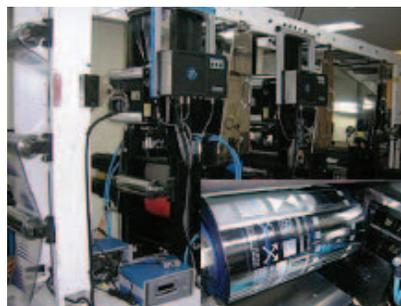
Roll-to-roll printed RFID
