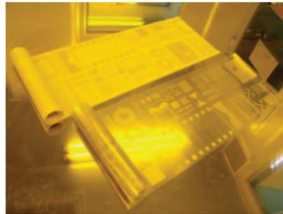
Roll-to-roll printed electronic devices
