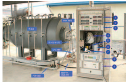
그림 7. 200,000kcal/hr combustor and reformer, ① ~ ③ : flow & temp. controller, ④ : reformer, ⑤ ~ ⑦ : water supplier, ⑧ : gas analyzer, ⑨ : power supply
