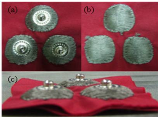
Figure 5. Original photograph of finished electrode. (a) Surface having snap button to be attached with transmitter, (b) surface to touch skin, (c) inflated surface of electrode
