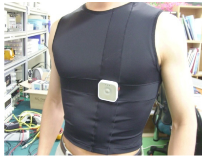
Figure 8. View on transmitter attached to clothing with electrodes
