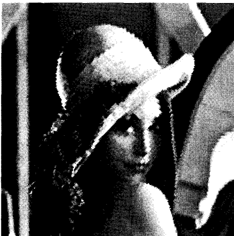
Fig. 5 Reverse recovery from the inverse log-polar map of the reverse image. The sub-sampling effect in the middle of the image is obvious
