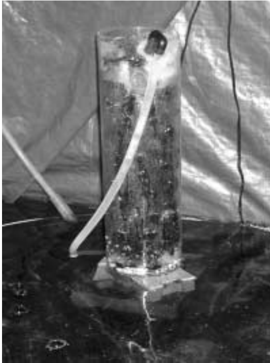
Fig. 3. Wet-dry filtering system.
