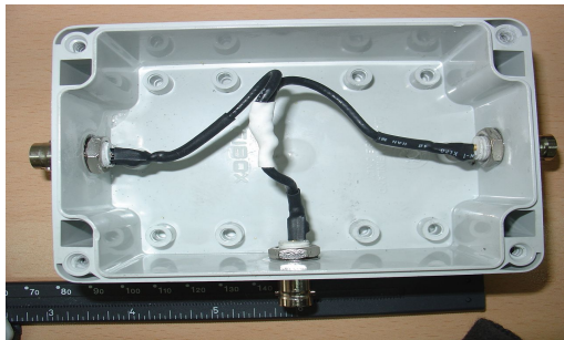
Fig. 3 Splitter for making shear wave on pyramid
