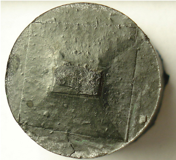
Fig. 3. Top view of Y1.5 sample with 15wt.% of BaCeO 3 addition.
