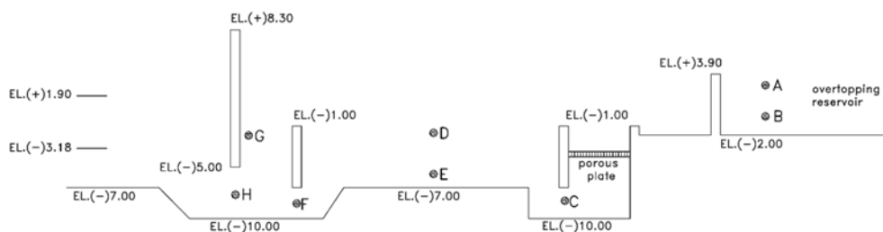
Fig. 1. Schematic diagram of the submerged outlet structure.
