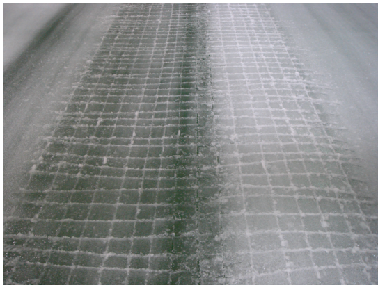
Fig. 4 Prepared brash ice
