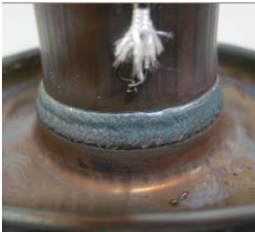
Fig. 12 No visible crack (bottom view)
