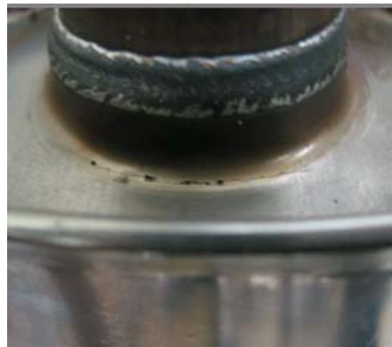
Fig. 9 Visible crack (bottom view)
