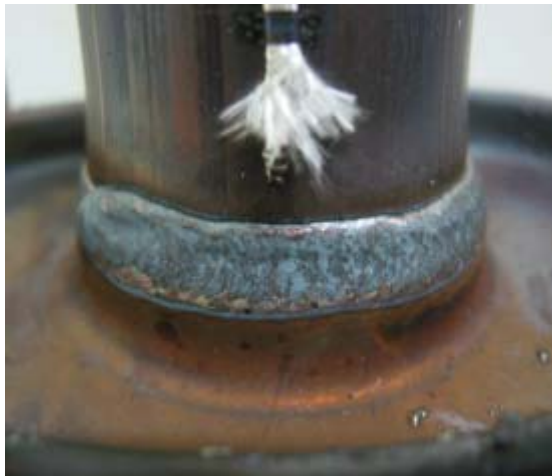
Fig. 11 Visible crack (top view)
