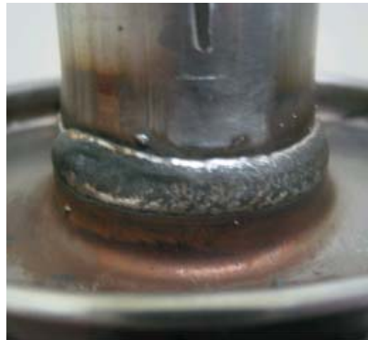
Fig. 8 No visible crack(top view)
