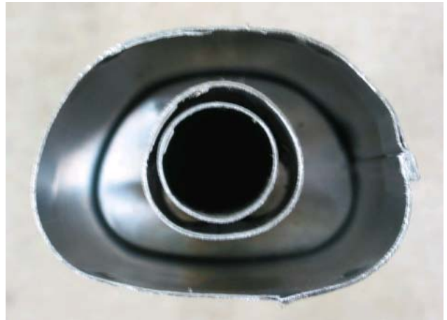
Fig. 2 Cut-away view of a resonator
