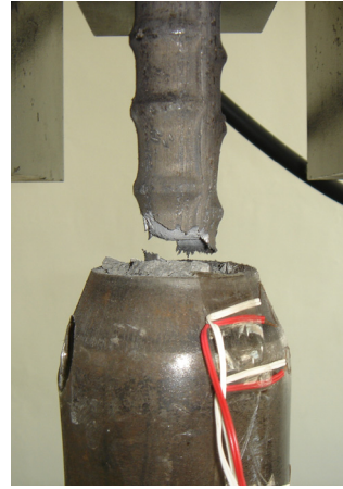
Figure 7. Final failure pattern (Specimen 37B2NC-1)
