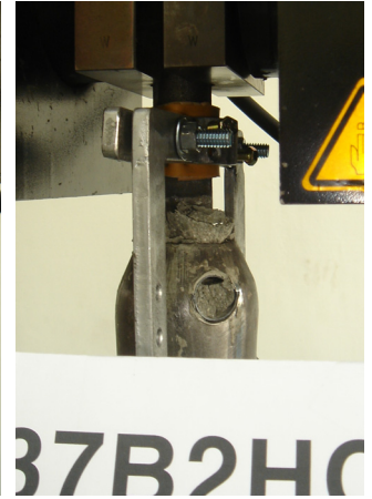
Figure 8. Final failure pattern (Specimen 37B2HC-1)
