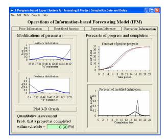
Figure 9. Forecasts of project progress and probability distribution on completion date during 6 Periods (30% completion)
