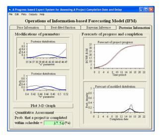
Figure 7. Forecasts of project progress and probability distribution on completion date during 2 Periods
