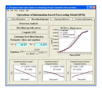
Figure 4. Determination of the best-fitted growth curve to the BCWS plan
