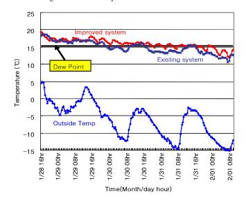
Figure 15. Surface temperature distribution of door
