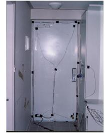
Figure 13. Measurement point of surface temperature
