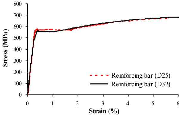
Figure 4. Stress-strain relationship of D25 and D32 bar
