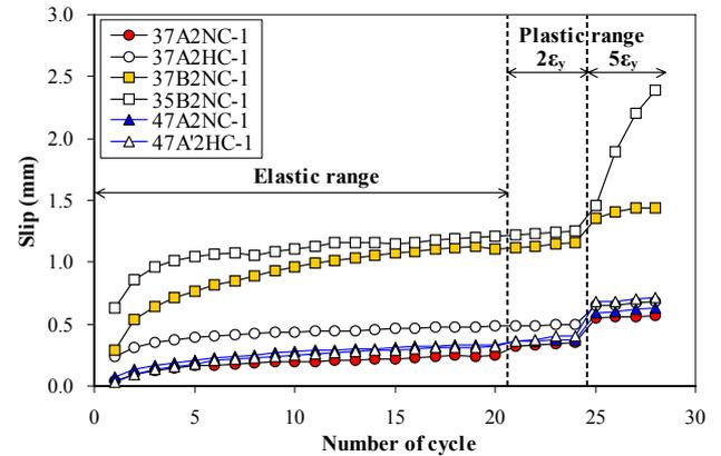
Figure 21. Change trend of plastic slip by cyclic loading on representative specimens
