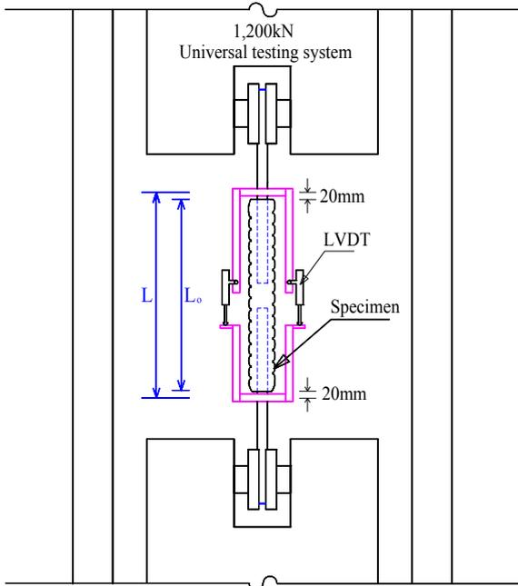
Figure 6. Specimen setup
