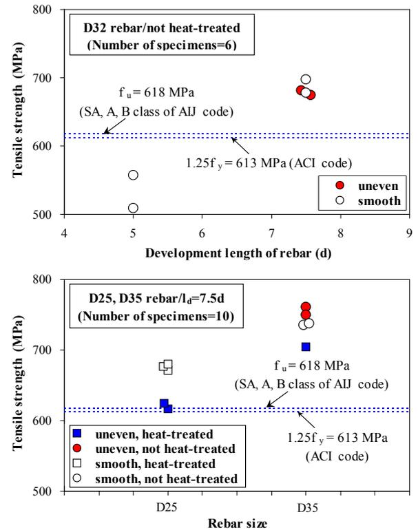
Figure 11. Comparison of tensile strength (sleeve type)
