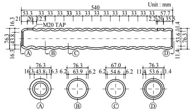
Figure 2. Details of A2 type uneven sleeve
