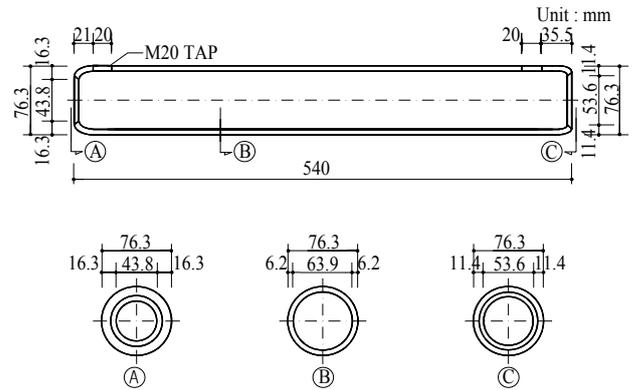
Figure 3. Details of B2 type smooth sleeve
