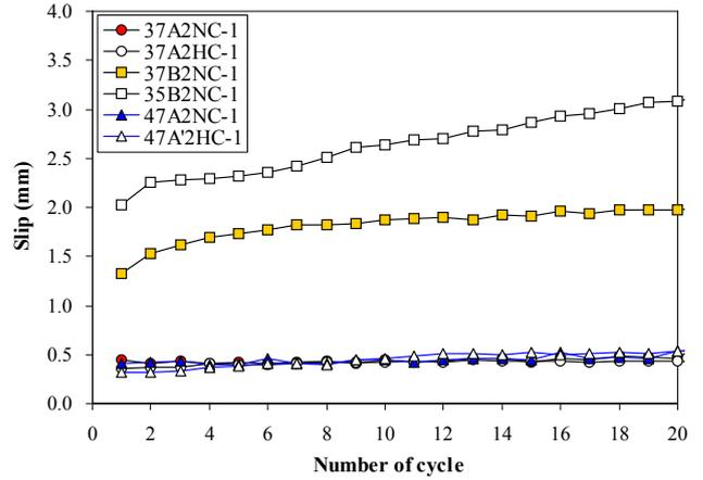
Figure 20. Change trend of elastic slip by cyclic loading on representative specimens
