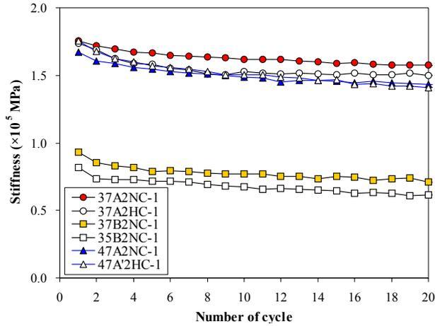
Figure 16. Stiffness change trend of representative specimens by cyclic loading
