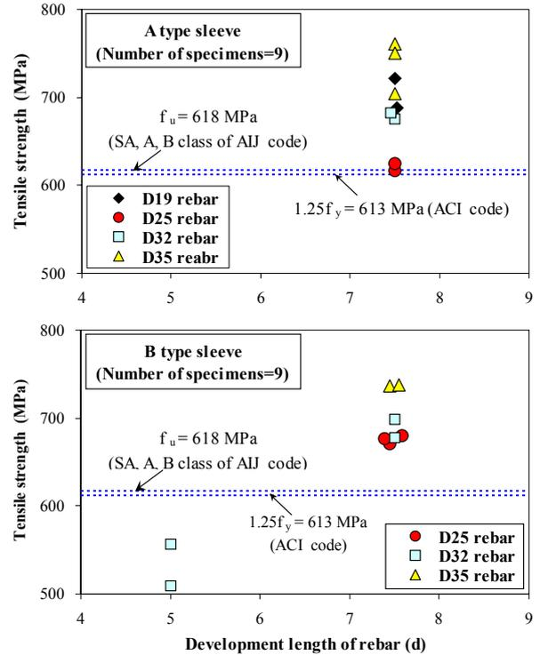
Figure 10. Comparison of tensile strength (rebar size)
