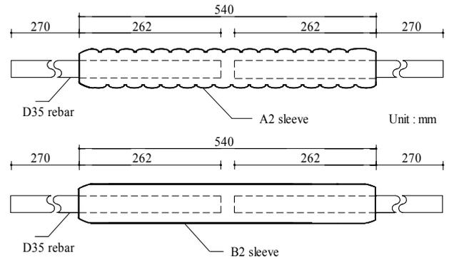
Figure 1. Representative test specimens (For D35 reinforcing bar, development length=7.5d)
