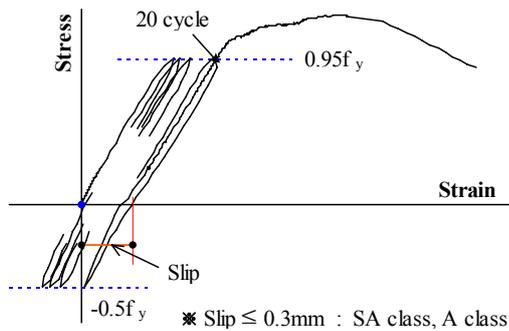
Figure 17. Definition of slip in elastic range (AIJ code)
