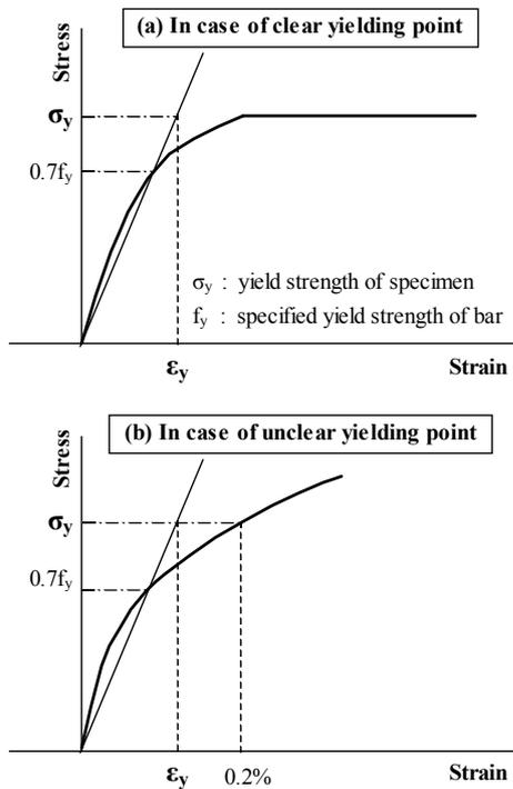
Figure 8. Definition of yield strain  $\epsilon_y$  of a specimen
