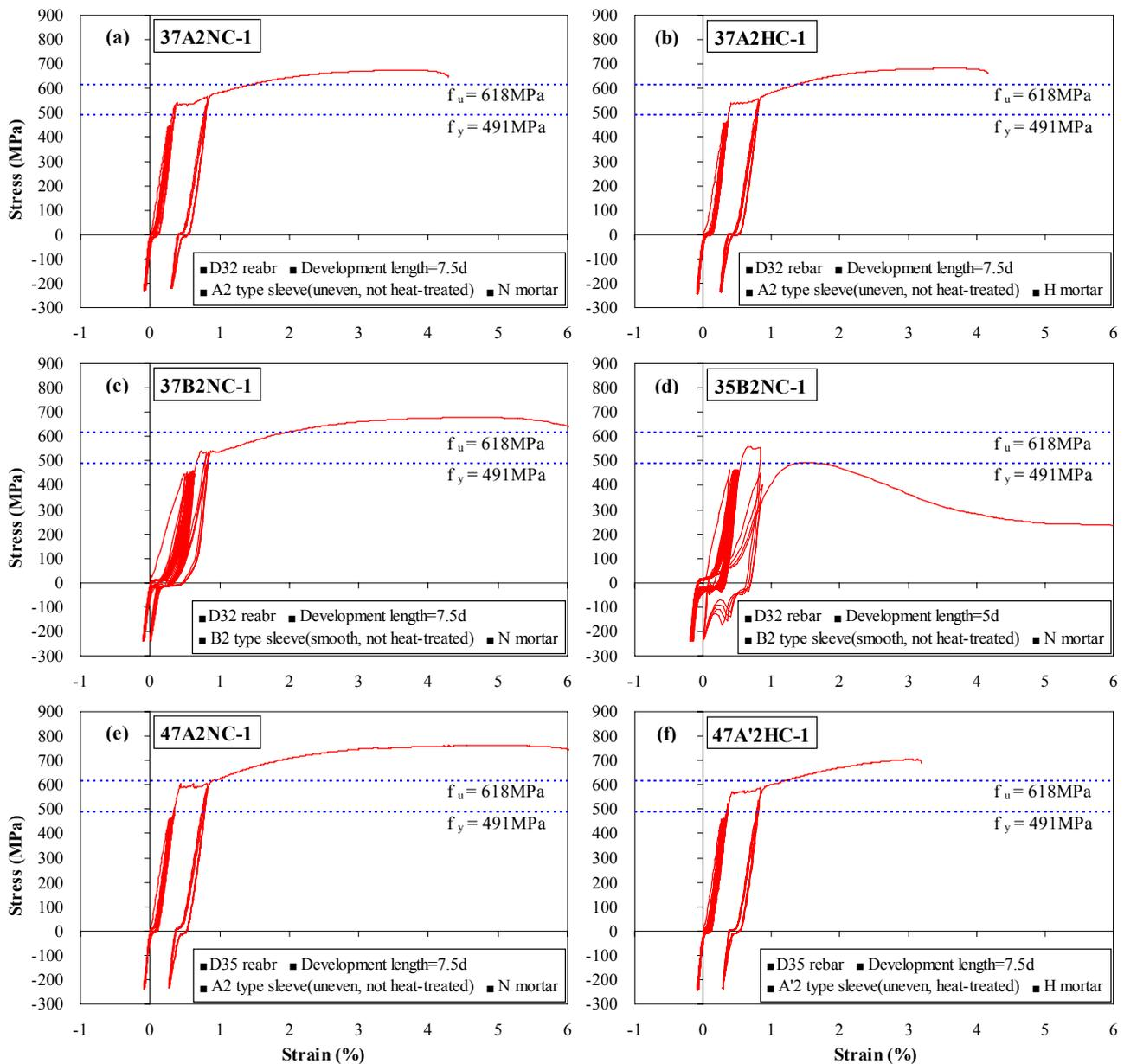
Figure 9. Stress-strain relationship of representative specimens
