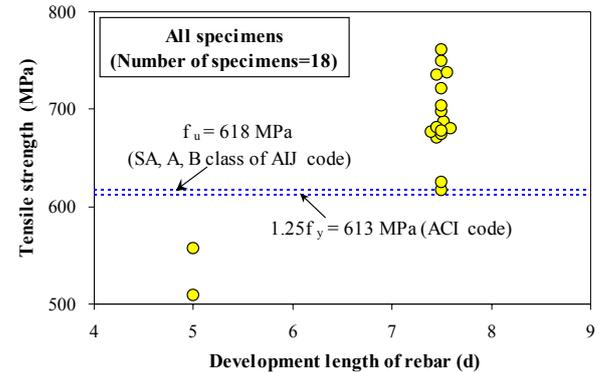
Figure 13. Comparison of tensile strength (all specimens)
