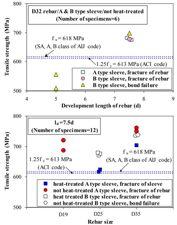
Figure 12. Comparison of tensile strength (final failure mode)
