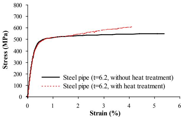
Figure 5. Stress-strain relationship of steel pipe with a thickness of 6.2mm
