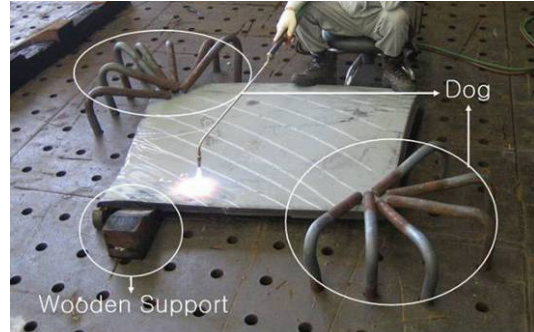
Fig. 8 "Dog" and "Wooden Support" (Park et al. 2007b)
