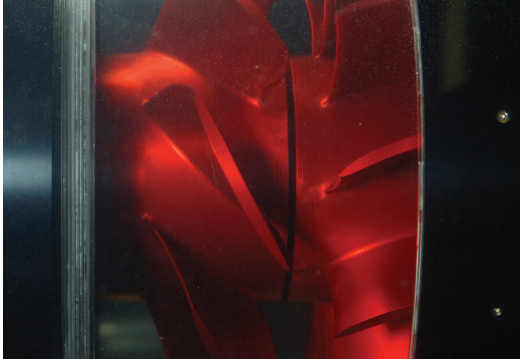
Fig. 6 Cavitation inception at J_Q=0.6988(\sigma_n=5.0)
