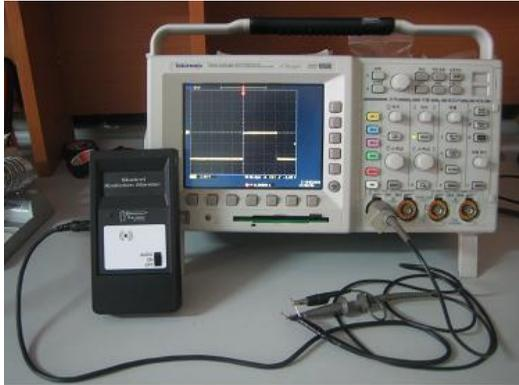
Fig. 2. Student Radiation Monitor used during tests.
