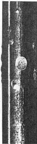
Fig. 13. Nodular corrosion on CANDU fuel element tested 90 days in INR TRIGA Reactor (x 1.5)
