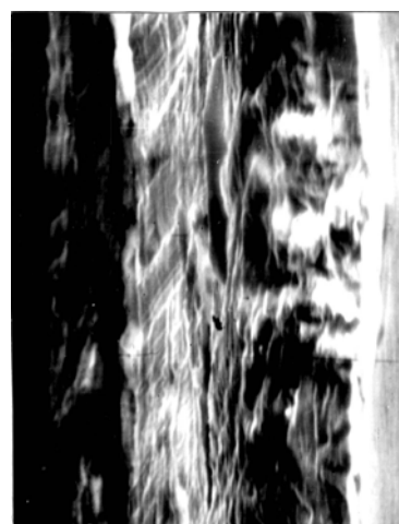
Fig. 2. Morphology of oxide film formed on Zr-2.5%Nb tested 30 days in LiOH- pH=12.5 (x1000)
