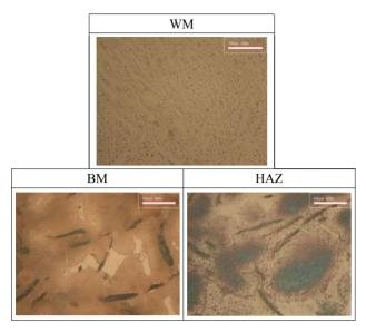
Fig. 8. Optical microstructures of HAZ, BM and WM (×600)
