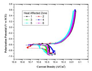
Fig. 5. Polarization curves of HAZ in sea water solution.
