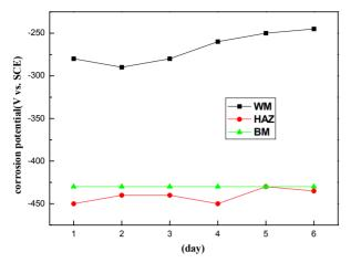
Fig. 3. Variation of corrosion potential in various area in natural sea water solution.
