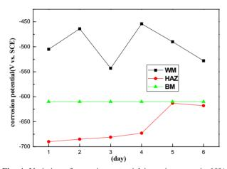
Fig. 4. Variation of corrosion potential in various area in 10% H<sub>2</sub>SO<sub>4</sub> solution.
