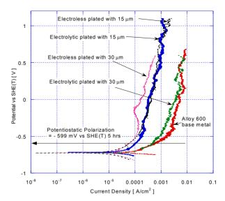
Fig. 5. Potentiodynamic polarization curves of Alloy 600 base metal and Ni-plated Alloy 600 in typical PWR water condition.
