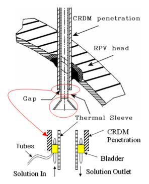
Fig. 10. Special end-effector using hydraulic bladder for remote electroless Ni-plating process in CRDM nozzles
