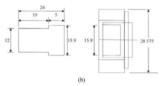
**Fig. 4.** (a) Photograph showing two locations of specimens installation in the flow accelerated corrosion experimental facility, and (b) drawing of specimen (left) and standard high pressure fitting (right)
