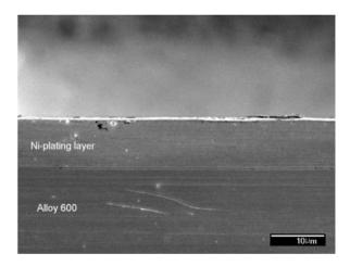
Fig. 9. Scanning electron micrograph of cross section of plate specimen after remote electroless Ni-plating
