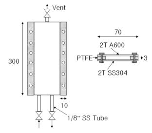
Fig. 8. A schematic design of plate specimen for remote electroless nickel-plating process to simulate the narrow gap between CRDM penetration and thermal sleeve
