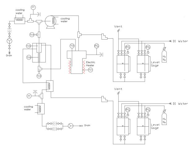
Fig. 3. Schematic of flow accelerated corrosion experimental facility in high temperature aqueous environment.
