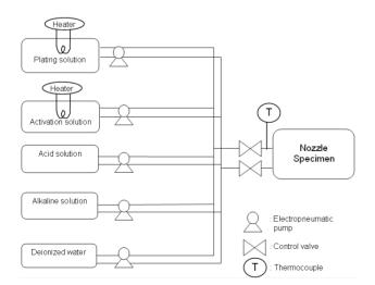
Fig. 7. Schematic of remote electroless nickel plating process.
