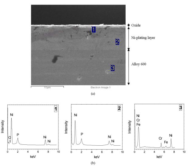
Fig. 6. (a) Scanning electron micrograph and (b) EDS measurements of nickel plated Alloy 600 specimen exposed to high temperature, high pressure and high flow-rate water with  $250^{\circ}$ C, 15 MPa and 2 meter per second for 20 days.
