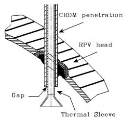
Fig. 1. CRDM nozzle on the reactor pressure vessel head in  $\ensuremath{\mathsf{PWR}}$
