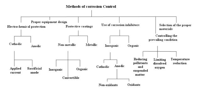
Fig. 3. Methods of Corrosion Control
