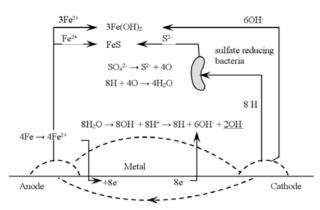
**Fig. 2.** Chemical reactions ending with ferrous sulfide and ferric hydroxide (corrosion products), where sulfate reducing bacteria play an active role.<sup>7)</sup>
