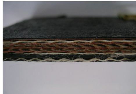
Fig 3. Section Crashworthy and Self-sealing Material for Designed Fuel Tank
