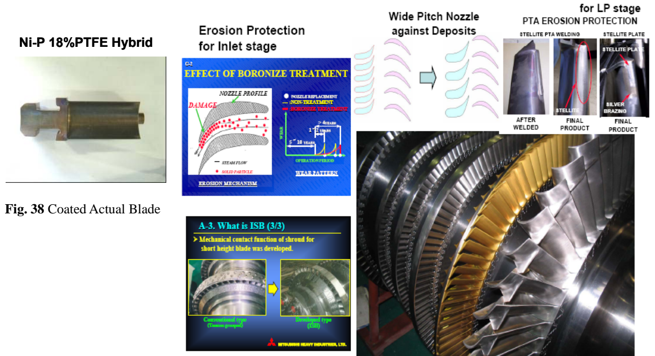
Fig. 39 Improvement of Blade Integrity, Coating Application of Actual Blades and Additional Improvement for Anti-efficiency deterioration
