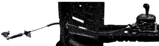
Fig. 2 Schematic of transmission cable(courtesy of KCW Co.)
