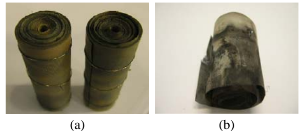
Fig. 9 Mesh-typed microchannel catalyst (a) before (b) aged
