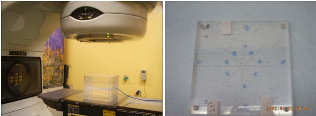
Fig. 4. Dose measurement of TLD in quality assurance of intensity modulated radiation therapy.
