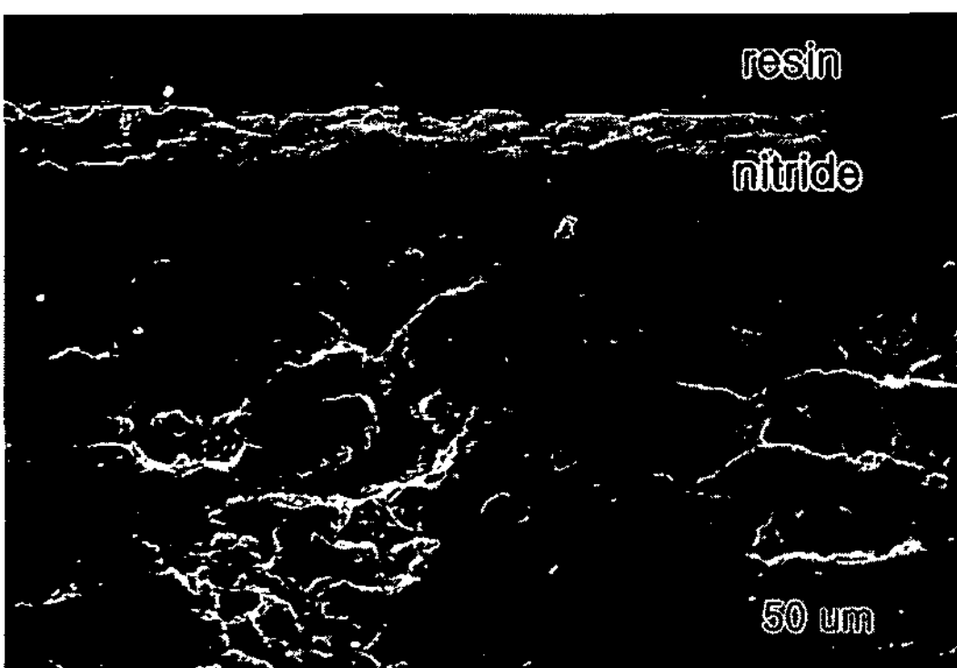
Fig. 5. A microstructure of a sintered nitride pellet fabricated by using SIMFUEL.
