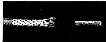
(a) Cable between high voltage battery and inverter
