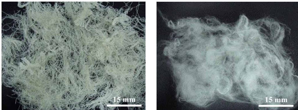
Figure 1. Views of waste wool fibers (left) and polypropylene fibers (right) used in this work.
