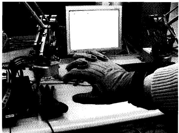
Fig. 2. A CyberGlove system for a human hand.
