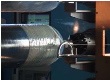
Fig. 2 Filament winding process of a fuel storage vessel
