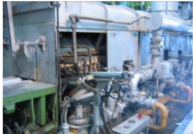
Fig. 2 High frequency preheating furnace using preheating of billet
