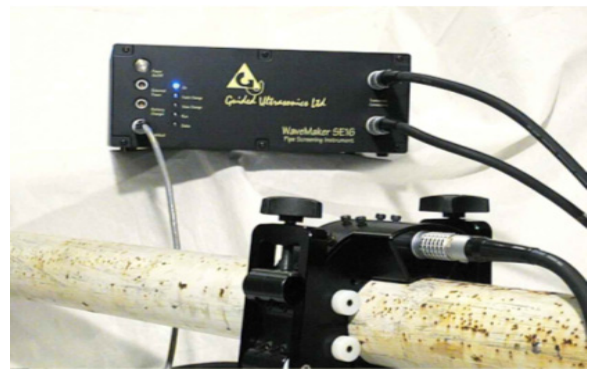
Fig. 7 Ultrasonic guided wave measuring system
