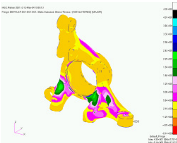
(c) Max. principal stress contour of 0.5GVW right & left
