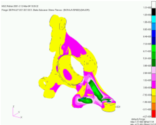
(b) Max. principal stress contour of 1.0GVW before & after
