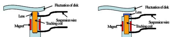
Fig. 7 Modify the moving part for manufacturing
