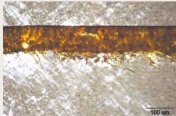
Fig 25. Polarized photo of body part of cylinder type lacquerware 5(x100)
