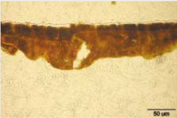
Fig 22. Transmitted photo of holed lacquerware(x200)
