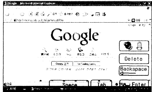
Fig. 2 A transparent window overlaid on the current desktop applications to get pen and voice input
