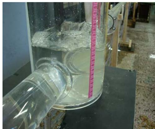
Fig. 8. Jet impact Phenomena by step height
