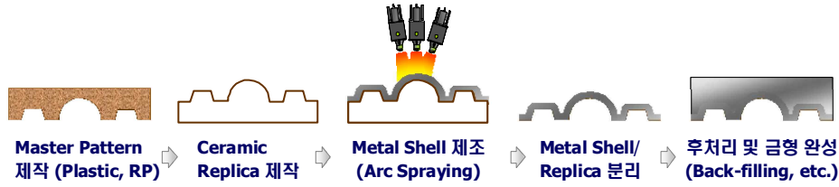
Fig. 3 Manufacturing process of die using high carbon steel
