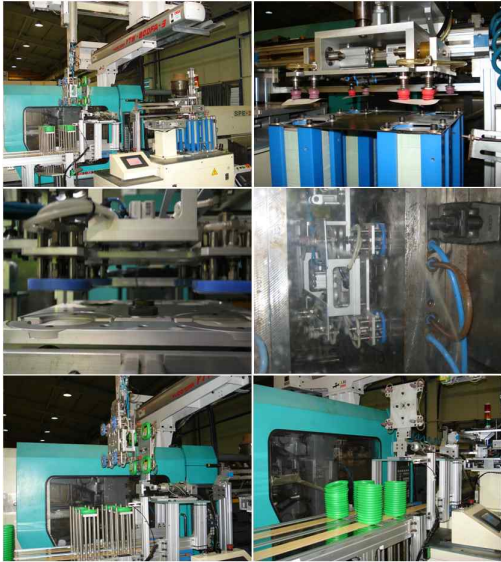
Fig. 10 Molding of rectangular 4cavity Flat-type IML parts
