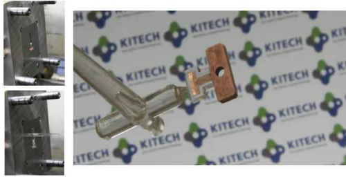
Fig. 7 Injection molding part (T-type, Gate Length 300 \mu m)
