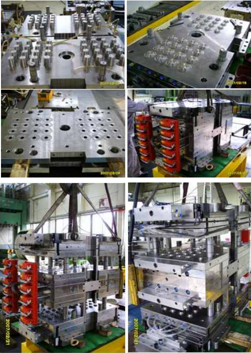
Fig. 8 Completed workpiece of 2Level stack mold (2Level x 32cavity)
