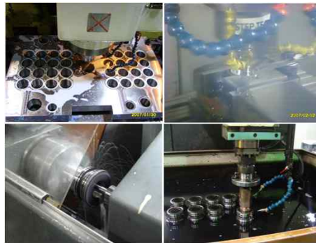
Fig. 6 Machining of parts for 2Level stack mold
