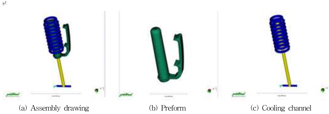
Fig. 5 FE modeling of preform and cooling channel
