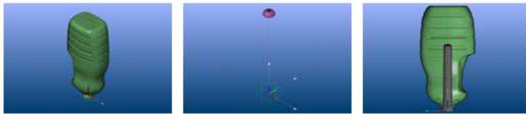
Fig. 2 FE modeling of blow molding
