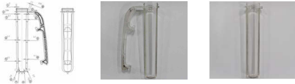
Fig. 7 Injection molding product and drawing of single body
